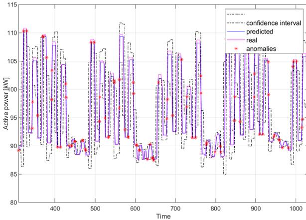
Figure 5: Real vs. predicted data (Building 1) - 95% confidence interval
