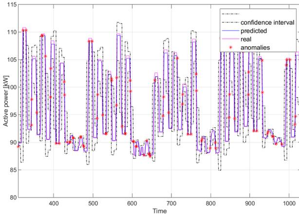
Figure 5: Real vs. predicted data (Building 1) - 95% confidence interval
