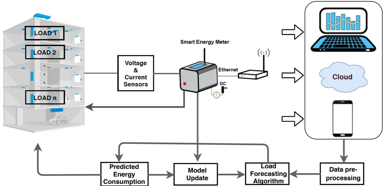
Figure 1: System architecture for electrical load monitoring
