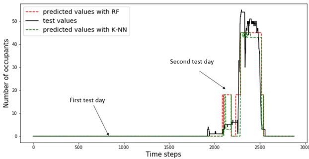
Fig. 6. Occupancy count for Room1 using RF versus K-NN with sliding window
