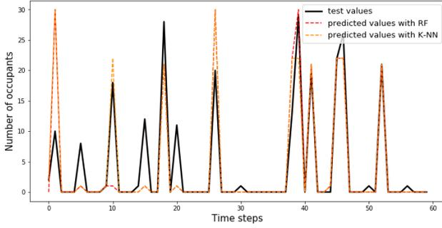
Fig. 5. Occupancy detection for Room4 using RF versus K-NN
