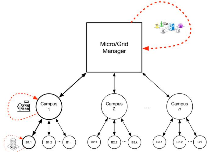
Fig. 1: Hierarchical energy system with three layers
