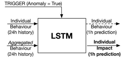
Fig. 4: Architecture of the anomaly impact model (LSTM)
