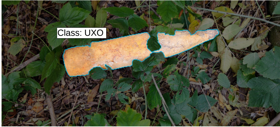
Fig. 1: UXO in the field can be oxidised, partially covered by vegetation/soil, and sometimes even component parts are missing, being difficult to use common retrieval approaches. The illustration is produced by running the Segment Anything Model [24] on the annotated bounding box of a UXO sample from the CTX-UXO dataset [8].
