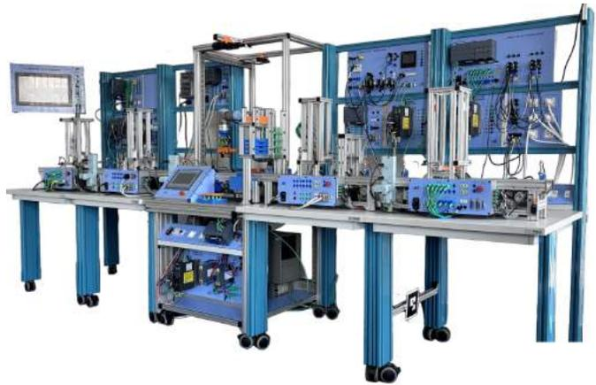
Fig. 1: Flexible Assembly Line System (FAL) for Smart Manufacturing
