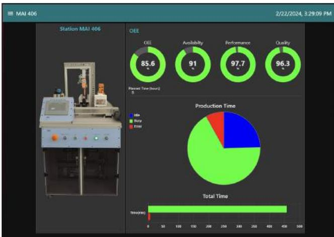
(b) Final inspection and rejection station
